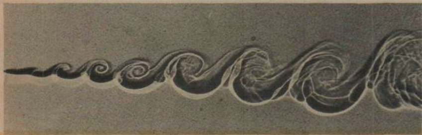
Figure 3 This modern laboratory photograph shows the type of structure formed by relatively slow-moving fluids (here helium and nitrogen gases). The wake is called two-dimensional because it is flat.
