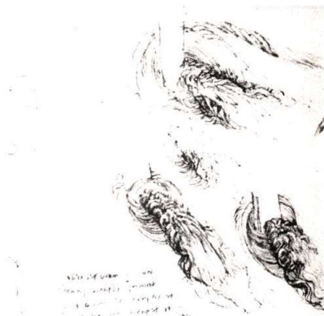
Figure 6 The experiments on this page of Leonardo's notebook show more complex wakes that are combinations of the two fundamental types. Leonardo says in his accompanying text that all fluid motion is "built up" out of the flat and braided kind of vortices.
