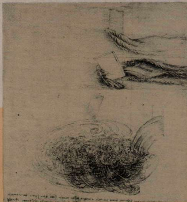
Figure 1 A page from Leonardo's notebook, showing the results of several experiments with water. The two smaller diagrams above show two kinds of wakes (flow) made as the water moves past an obstacle. The lower diagram shows the complex wake made by a jet of water pouring into a pool of unmoving water.
