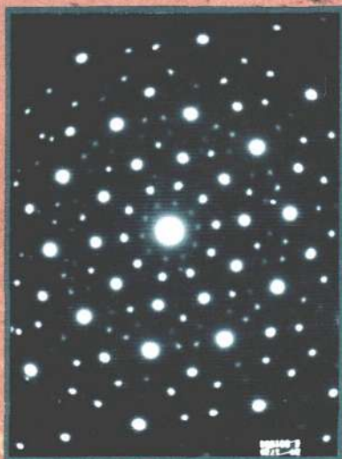
Courtesy of D. Shechtman A computer-enhanced image of pentagonal diffraction patterns formed by exposing aluminum-manganese crystals to Röntgen rays.
