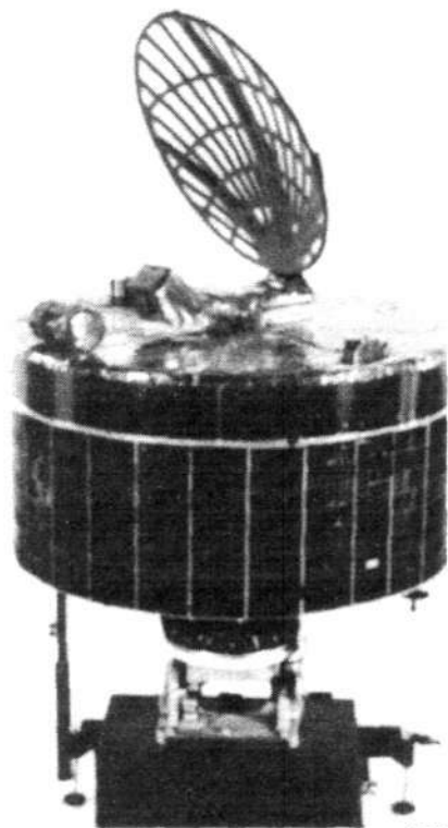
ISAS Japan's Suisei spacecraft, launched by the Japan Institute of Space and Astronautical Science Aug. 19, 1985, carried an ultraviolet telescope and an analyzer to measure the energy and direction of electrons and ions in the solar wind.
