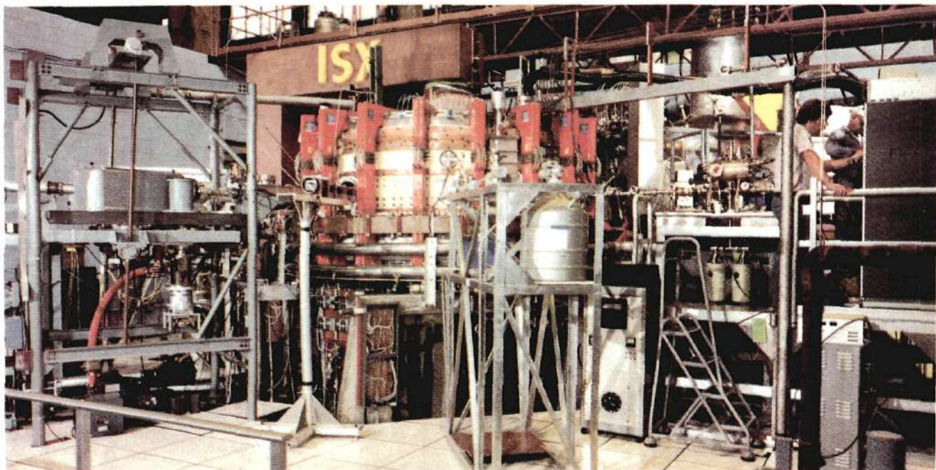
The ISX tokamak at the Oak Ridge National Laboratory showing the neutral beam heating apparatus. ORNL made the neutral beam equipment for the PLT tokamak at Princeton Plasma Physics Laboratory, which achieved record temperatures in August 1978.
