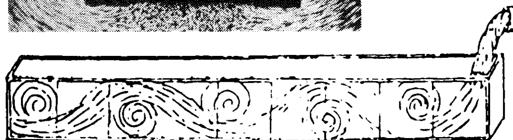
▲ Drawn by Leonardo, this vortex structure is today known as the van Karman "vortex street" which forms in the wake of a moving airplane.
