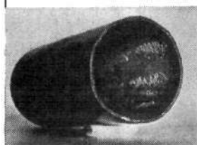
AFTER: After continual treatment most scale is removed and will be prevented as long as the system is in operation.
