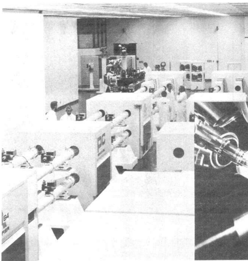
The Omega laser system: 20 times the entire electrical generating capacity of the United States. Inset is an inside view of the target chamber showing the target support stalk, focusing lenses, and diagnostic systems.
