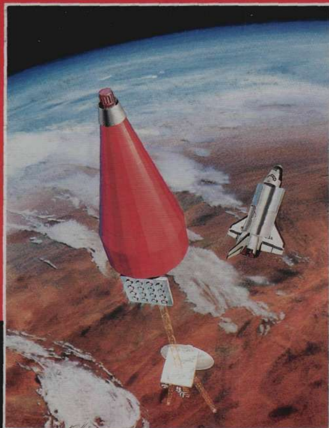
Artist's depiction of an SP-100 space nuclear power station attached to a Galileo-type spacecraft launched by the Space Shuttle and destined for Neptune.
