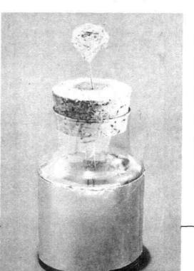
The Leyden jar is a capacitor or condenser that stores electrical charge. The charge is stored on the inner surface of the glass and induces an opposite charge on the outer surface. The glass is a dielectric; that is, a charge cannot pass through it until a certain high level of charge has accumulated. The purpose of the inner and outer layers of foil is to conduct and distribute the charges over the two surfaces of the glass.
