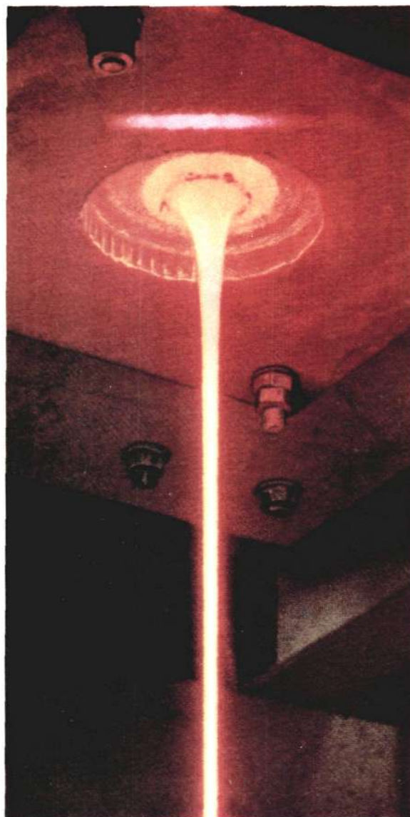
Production of vitrified waste at Marcoule, France. CEA
