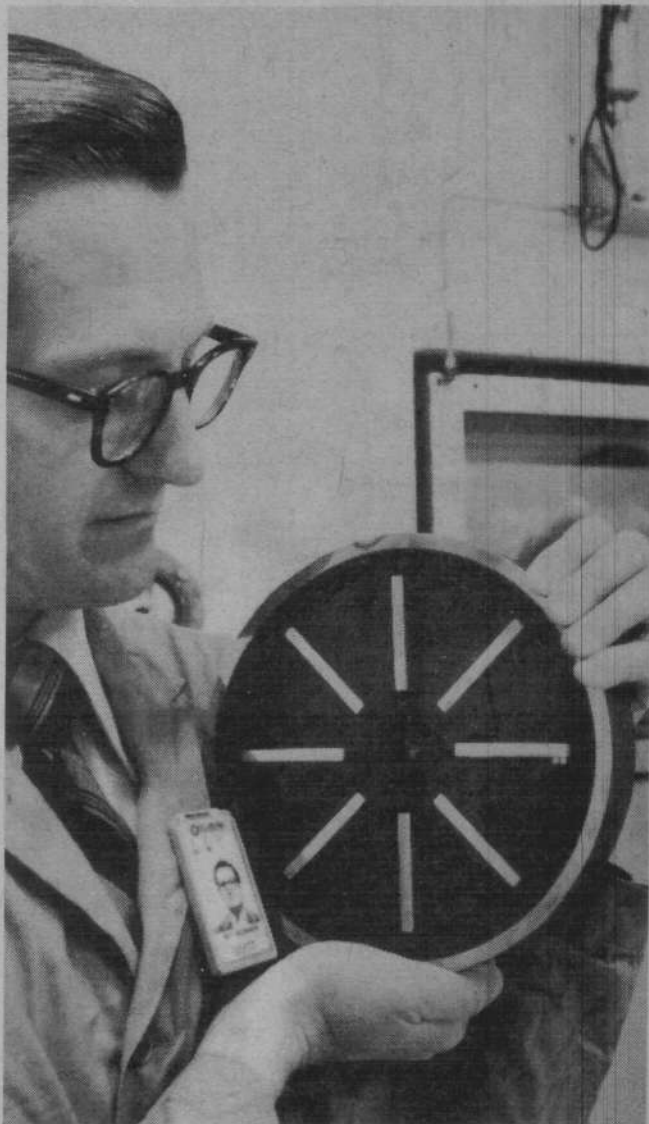
A cross-section view of high-level waste glass test material solidified in a steel waste canister is displayed here by William Bonner, the technical leader of nuclear waste processing at Battelle's Pacific Northwest Laboratories.
